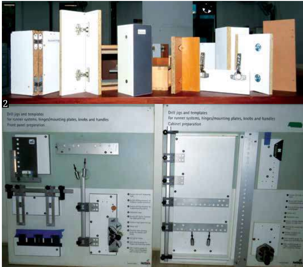
2 Hinges, sliding systems, knobs and handles need expert preparation in boring and drilling, ahead of installation.
